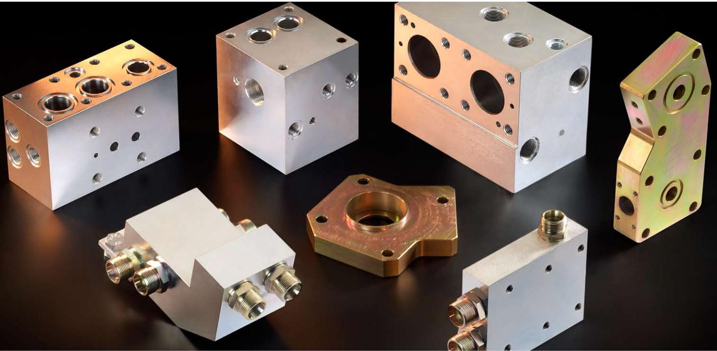
Purge valve blocks of VB 16 series are used in hydraulic closed loop circuits with motors in which a purge valve is not installed (e.g. circuits with radial piston motors). They serve for circuit flushing, reducing temperature in the system and removing air from hydraulic fluid.
