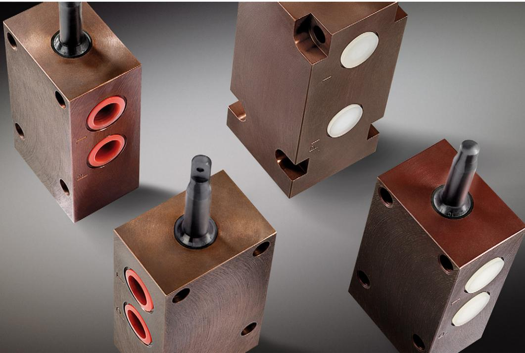
Inch valves are used in hydrostatic propel systems of mobile machines as an override control of variable pump. In such systems, in which variable pump with speed-dependent control are usually used, inch valve serves for braking or quick stop and for slow smooth take-off of the machine when the pump main control is not in function.
